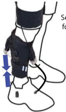
Sensors on each foot detect gait events and synchronize timing of assistance
